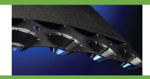
Rigid drainage board manufactured from HDPE. Combined function as a water-retention, drainage and filtration layer. Rigid sheet with integrated Polypropylene filter layer. Studded HDPE sheets contains perforations to drain surplus water and high capacity dimples (height c.20mm) for water retention. High compressive strength (115kPa). Delivery and installation according to Grey2Green instruction. Product arrives in two different sizes, 48.5 m2 and 24.25 m2.
